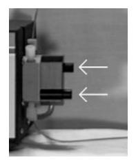
Figure 2-1. Flow Cell Thumbscrew Locations
