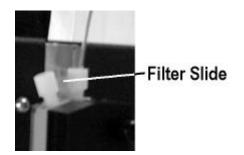
Figure 3-1. Filter Slide Location
