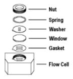
Figure 5-1. Flow Cell Window Assembly
